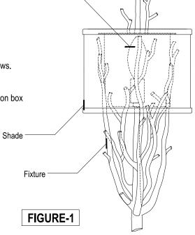
3. Fasten the white fixture lead to the white wire in the junction box. Fasten the wires together with an approved fastener (wire nut). Starting about 1" below the fastener, tightly wrap the connection with electrical tape so that the connections seals the end of the fastener.
